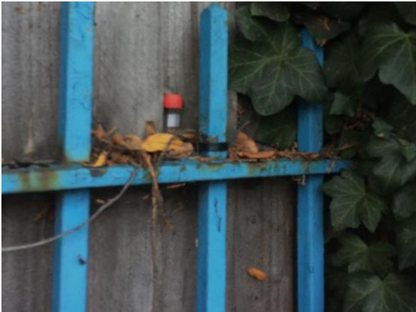
Diffusion Tube on day care centre playground fence on Romford Road
